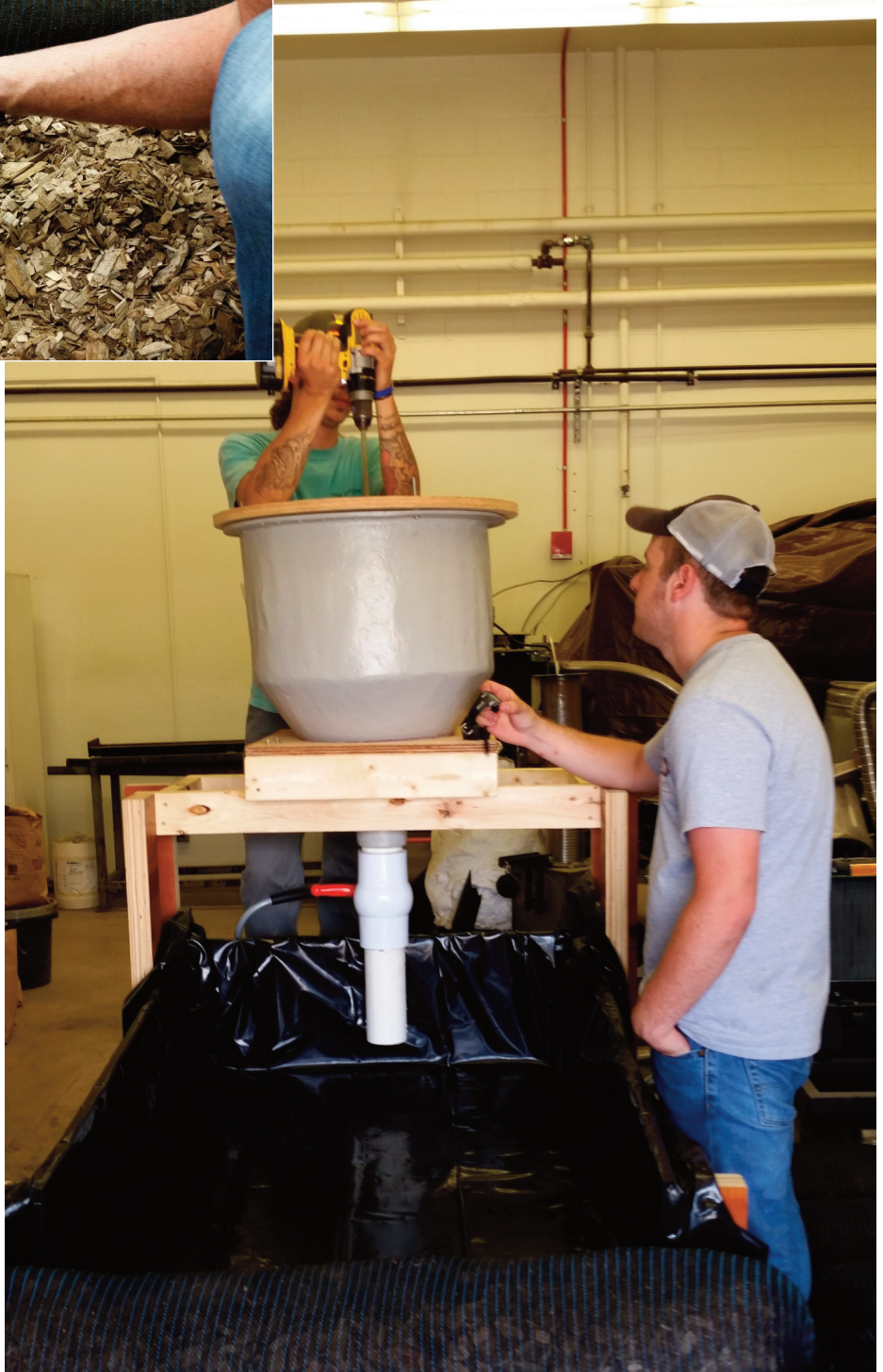
Undergraduate Research assistants operating silt sock testing apparatus
